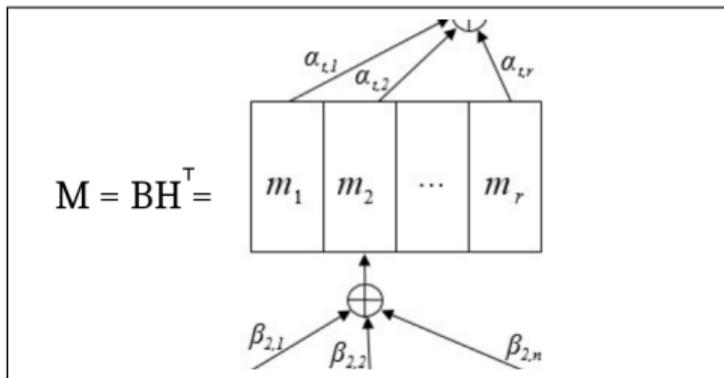
Figure 4: Zoom of the attention bridge in the compound architecture
